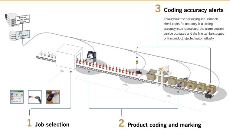
The product or appropriate code can be selected at the CLARiSUITE-installed PC or Videojet printer. Or, a bar code can be scanned from a work order or from the product itself with a hand-scanner. Information such as date/place of manufacture, best-before date, lot/batch number and a wide range of both production and consumer information is accurately applied to every product.
